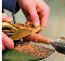
Take it for a spin. A block plane can be used on the lathe to achieve smooth, straight cylinders.
